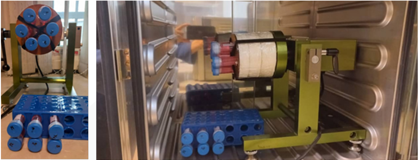
Figure 1. The clinostat used in this experiment and the placement of samples under microgravity (MG) and normal gravity (1G) conditions.
